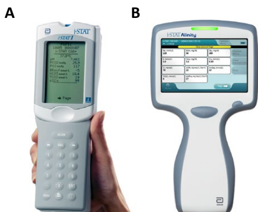
Figure 1: The Abbott Point of Care (A) iSTAT ® portable analyser system and (B) iSTAT Alinity ® portable analyser system. To be used in conjunction with either a Glucose or Chem8 cartridge for blood glucose concentration determination.
