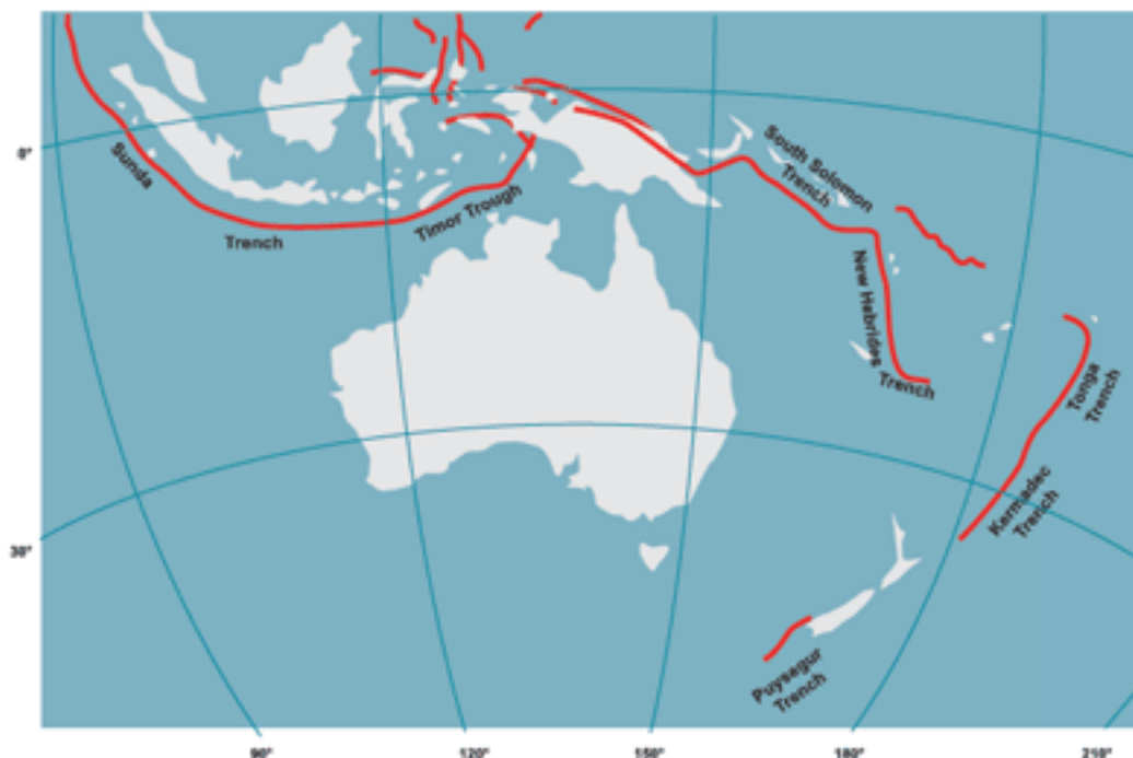
Figure 5 Subduction zones along tectonic plate boundaries (shown in red) surrounding Australia. These zones have the potential to generate a tsunami that may impact on Australia's coast. Source: Geoscience Australia; available at www.bom.gov.au/tsunami/about/atws.shtml
