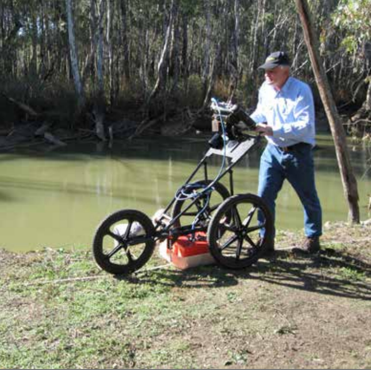
Use of Ground Penetrating Radar (GPR) (NPWS 2018)
