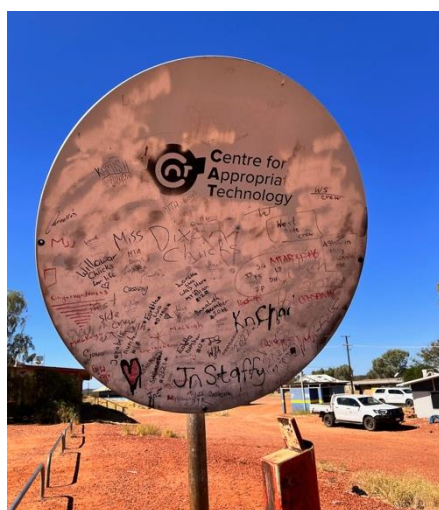
Figure 4: The CfAT HotSpot enables access to mobile signal from Yuendumu 43km away
