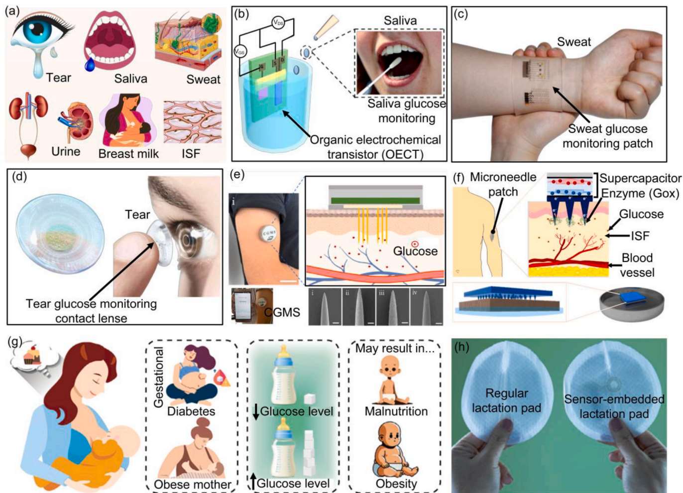
Fig. 1. Non-invasive glucose monitoring using alternative biofluids. (a) Tear, saliva, sweat, and urine offer pain-free alternatives to blood sampling for glucose monitoring. (b) Saliva-based sensors, such as organic electrochemical transistors (OECTs), enable non-invasive detection but are affected by pH variability. (c) Sweat glucose monitoring patches provide continuous tracking but depend on consistent sweat secretion. (d) SCLs detect glucose in tear fluid with high sensitivity, though challenges remain in accuracy and user comfort. Urine glucose testing (a) helps detect hyperglycemia but lacks real-time capability. Advances in nanotechnology, wearables, and wireless communication are enhancing sensor performance, usability, and accessibility for diabetes management. (e, f) Concept of a wearable glucose sensor system based on differential microneedles and its subcomponents, and a self-powered supercapacitor as a glucose sensor. (g) The importance of monitoring glucose in breast milk due to the potential impact of hypoglycemia and hyperglycemia on infant health, Reproduced with permission from Ref. (Al-Shami et al., 2025), 2025, Wiley. (h) Real photo of a commercial regular lactation pad and a sensor-embedded lactation pad, Reproduced with permission from Ref. (Al-Shami et al., 2025), 2025, Wiley.
